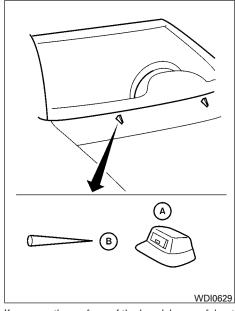
If you wax the surface of the hood, be careful not to let wax get into the washer nozzle (a). This may cause clogging or improper windshield washer operation. If wax gets into the nozzle, remove it with a needle or small pin (a).
